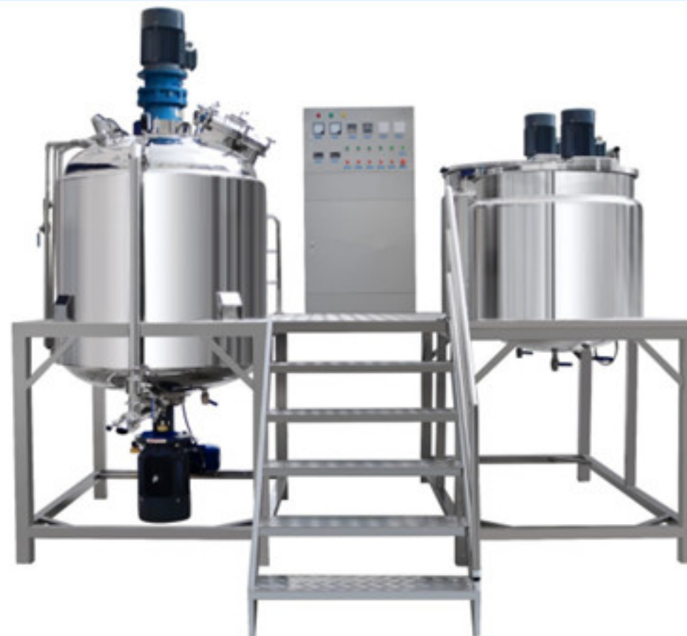
RHJ-D-500L Int & ext Circulation homogenizer
